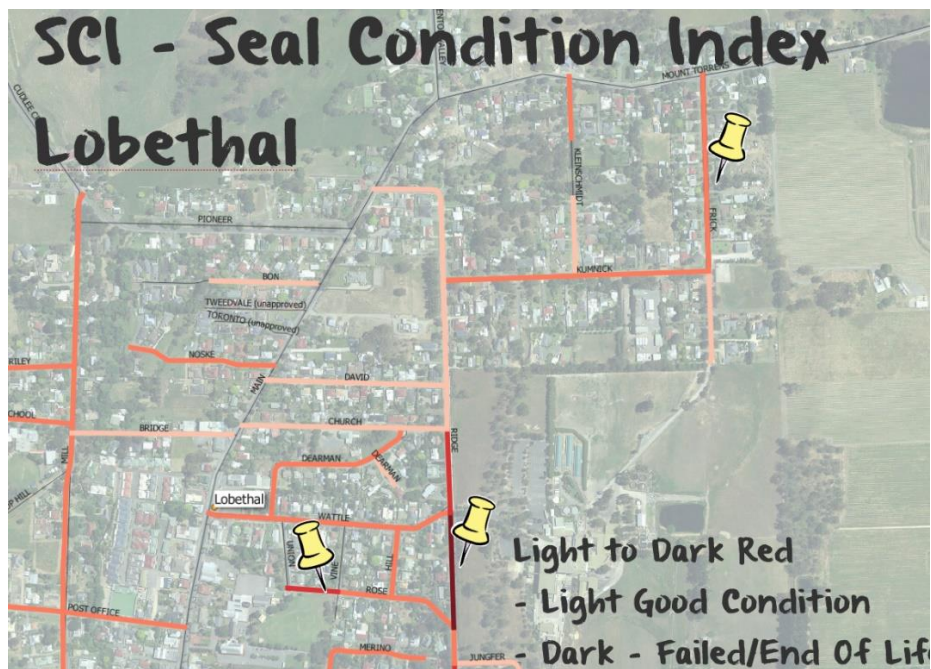
Lobethal – Seal Condition across each road based on the High Speed Data Collection.
