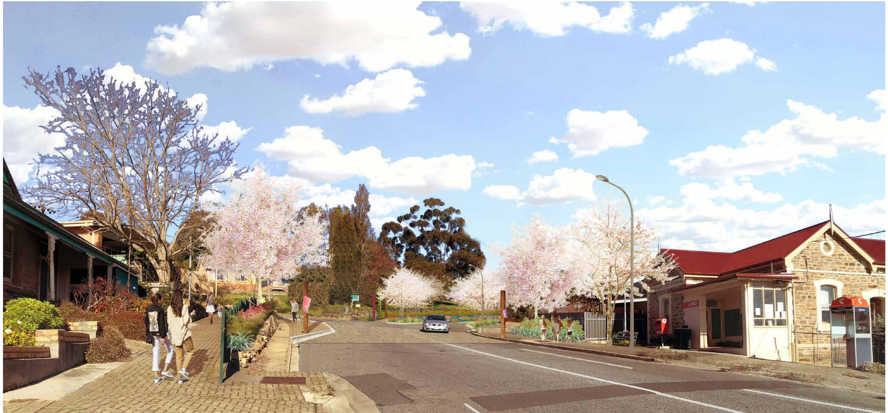
After - Artist's Impression: Paved build outs, unique marker signs and rumble strips to slow traffic and denote an entrance to the "Village Heart". Note : Image depicts street after power undergrounding and streetlight installation
