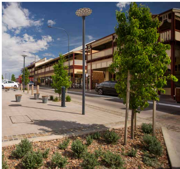
At Sixth Street, Murray Bridge, Jensen PLUS led a team to transform the streetscape into an attractive, green and functional street. Rain gardens pictured here catch stormwater and passively irrigate the new trees and plantings.
