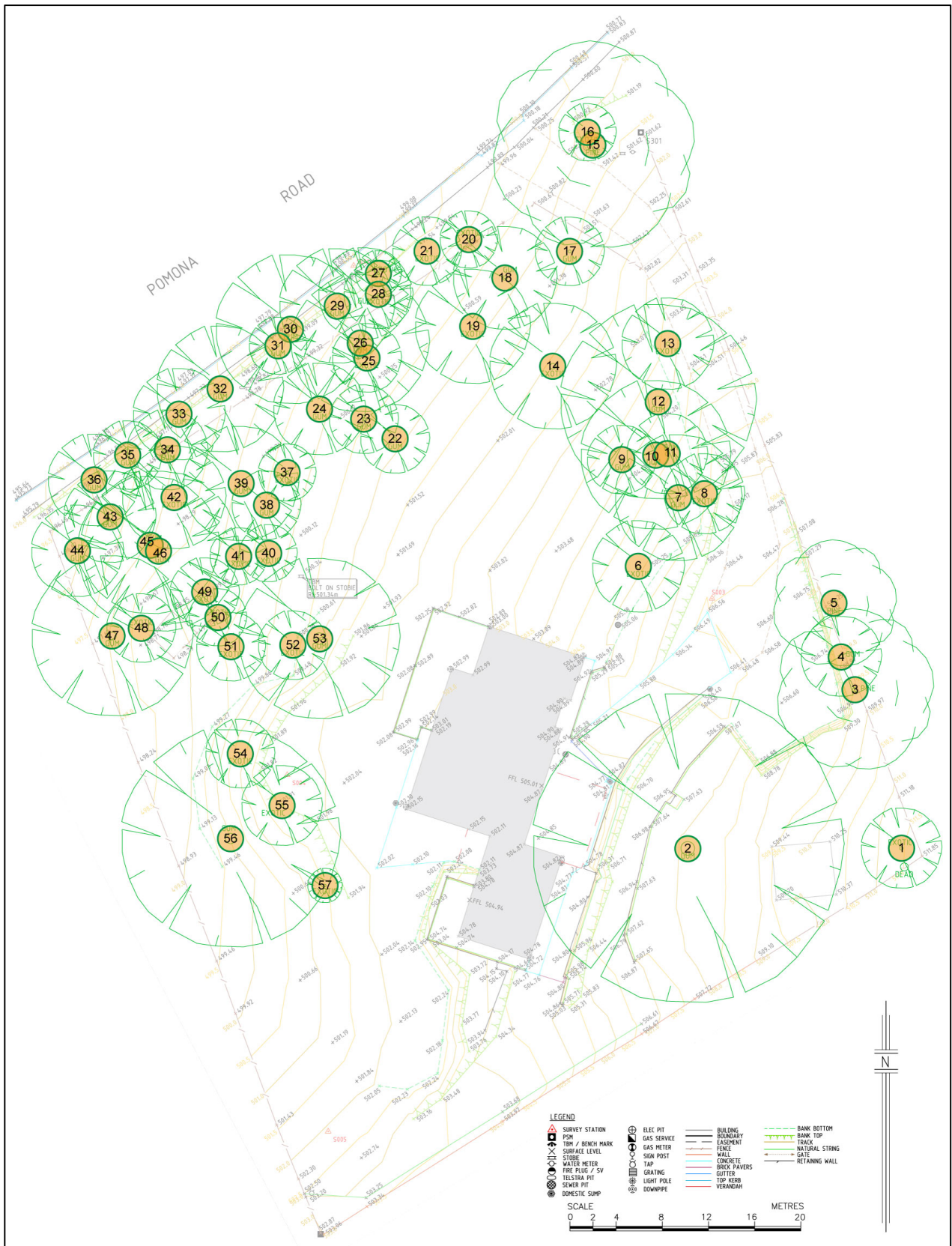
Figure 1. Site Plan. Extract from survey plan of the subject site (Michael Gear Surveys), indicating the location and labelling of the 57 trees included in my February 2018 arboricultural assessment. Trees 2, 6, 12 and 13 are no longer present on the site.
