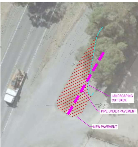
Figure 5: Proposed minor widening of the service road
