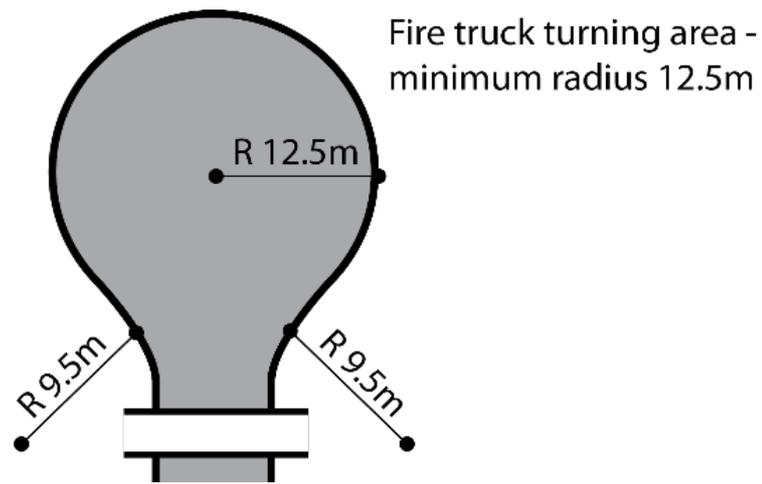
Figure 4 - 'T' or 'Y' Shaped Turning Head
