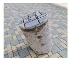
Figure 5: 25m Pool Floor Core 1
