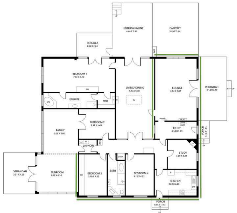
Figure 11 – Floor plan of former Coach House [Source: Real Estate 2022]; additions by author to show visible internal and external masonry walls (green line)
