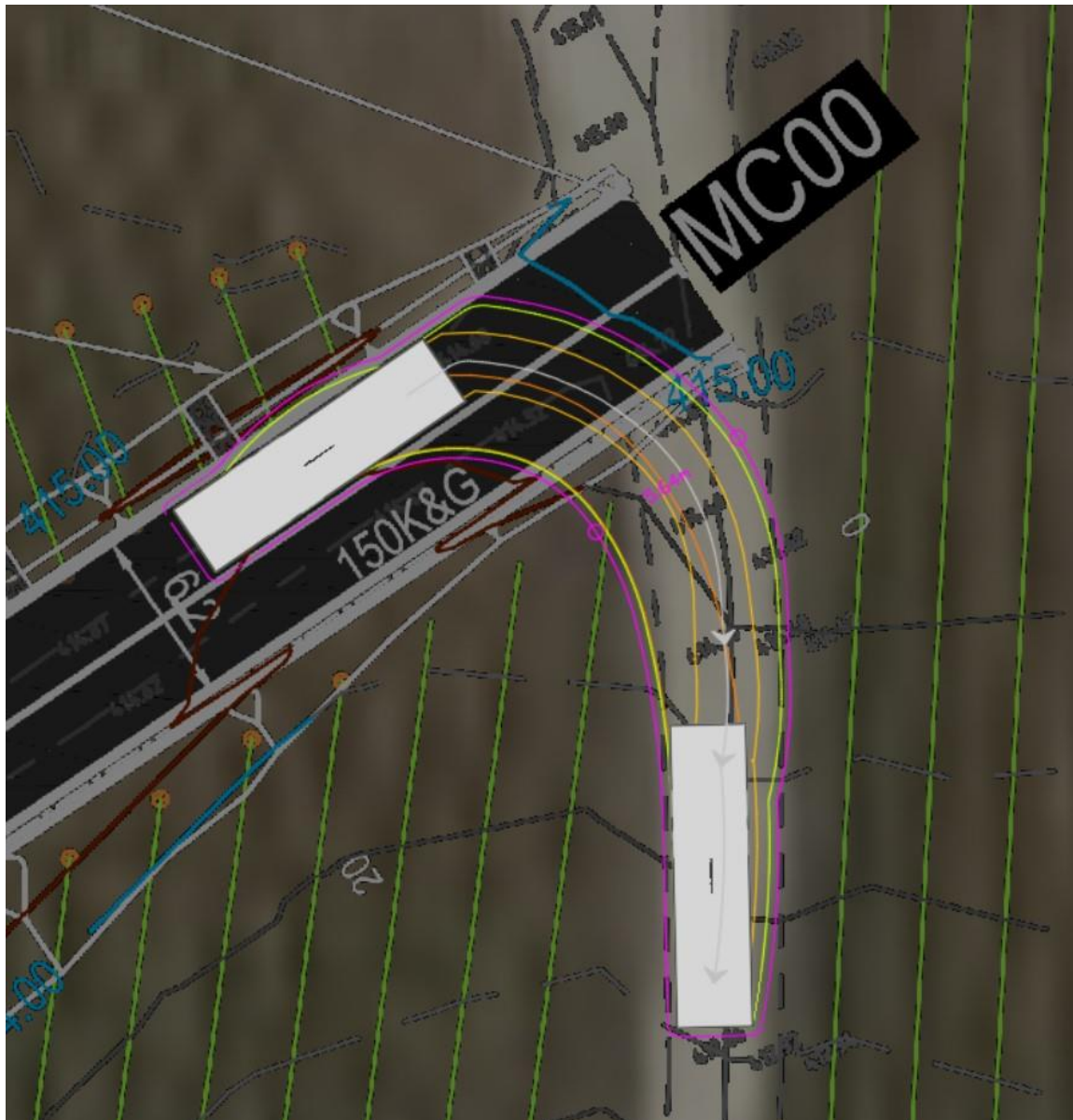
Figure 2: Swept path of a CFS Appliance
